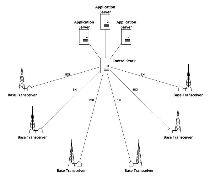
The M220X series base transceiver is designed to operate as part of an <u>locast</u> network. locast networks include a *control stack*, one or more *base transceivers* (such as the M220X), and tens to millions of remote *nodes*. Generally, base transceivers provide a sector of coverage, or part of a sector, and communicate with the control stack using the BXI interface.
